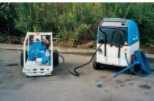
Together with the Dynabox 350, the trollies are truly hot-water washers using water of up to 130° C.
