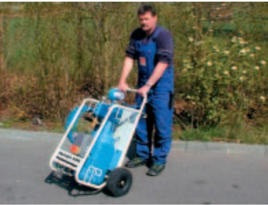
Contrary to twin-axle models, the Dynajet trolley need not be lifted but can be pushed and pulled along everywhere – even up and down steps.
