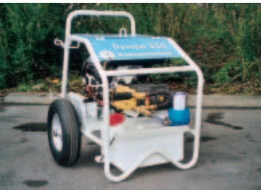
High performance even in the smallest space. The powerful 16 kW petrol motor can be started easily with an electric switch.
