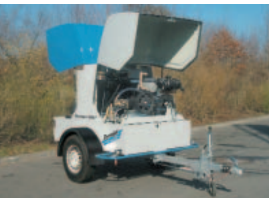
The heart of the Dynajet 500 th : a robust 32 KW diesel engine and the high-performance combustor.
