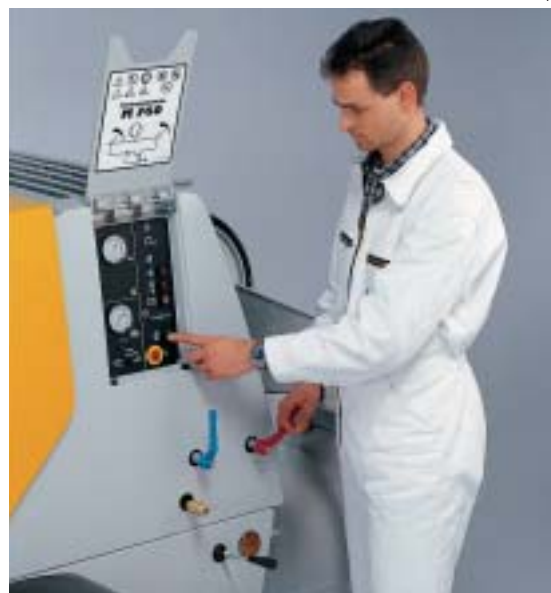
The control panel is protected by a red flap against dirt and damage.
