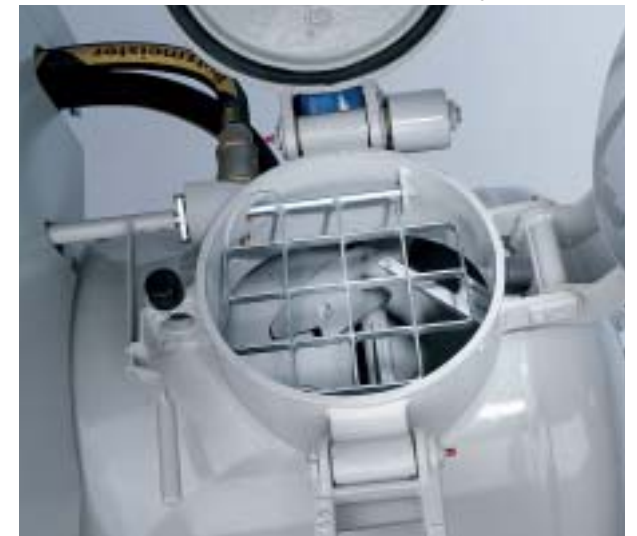
The M 760 is in keeping with all the valid safety regulations. When you open the hood the engine switches off immediately. This is also true by the way when you open the protective grid of the mixer.
